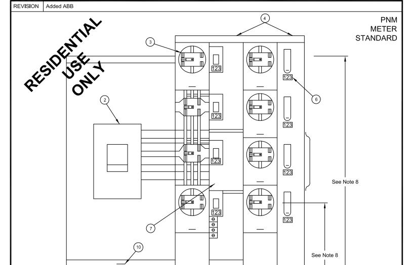
(1) Line duct must be rigid galvanized, Schedule 80 PVC or IMC. Coordinate size and number of line ducts with PNM.(2) Main disconnect may be required on the line side of any group of more than six
